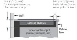
WARNING: INSUFFICIENT VENTILATION BETWEEN THE COOKTOP AND OBJECTS BENEATH IT MAY CAUSE A FIRE HAZARD.
