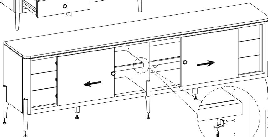
Adjust the leveler when necessary
