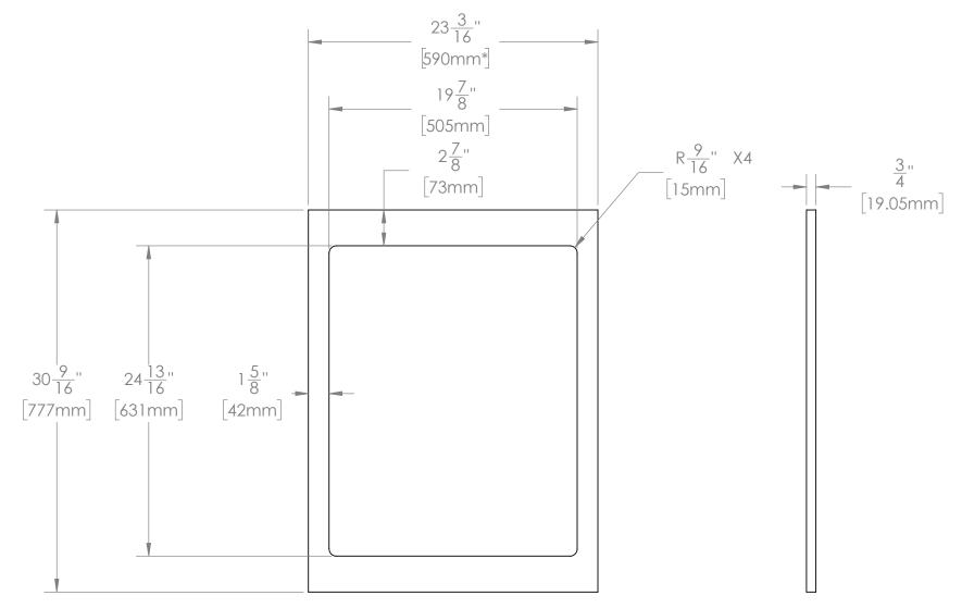
It is recommended the panel to be 590mm width but +/- 1mm tolerance is acceptable. Also, the aluminum frame can accommodate 5/8" thick panels as well, but will require shorter screws. Please discuss with your installer
