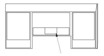
To install the hood with a duct, you will need to provide a hole for the duct. Please use the template provided to correctly place the hole.
