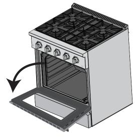
Lift up and pull the small levers located on the two hinges all the way back to unlock.
