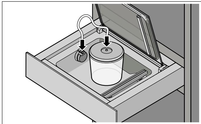
2. Plug the vacuuming adapter into the air outlet.
