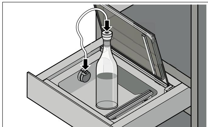
3. Secure the hose to the vacuuming adapter and the bottle adapter.
