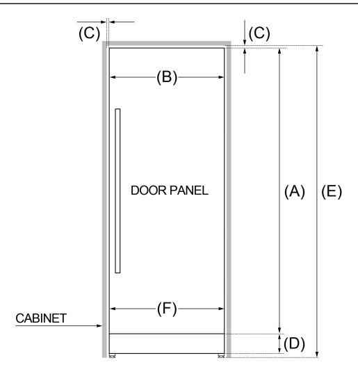
NOTE: The refrigerator comes with a 4" (100 mm) stainless steel toe kick installed to fit a standard 84" (2134 mm) tall cabinet niche.
