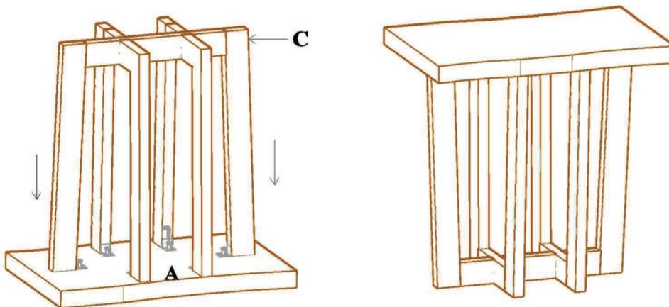
**TIGHTEN ALL BOLTS FIRMLY AT THIS TIME USING ALLEN KEY (E). SET END TABLE UPRIGHT.**
