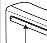
**DO NOT block** or obstruct the flow of air through the ventilation openings. The oven vent is located at the back of the appliance. The vents need to be unobstructed and open to provide necessary airflow that is important for proper oven performance.
