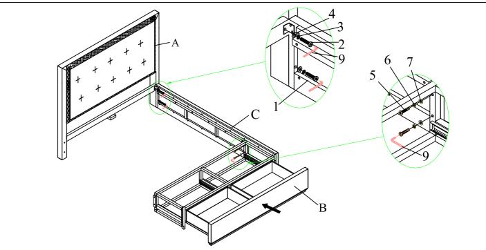
STEP 1: FOLLOWING THE ILLUSTRATION, ATTACH ONE SIDE RAIL (C) TO THE HEADBOARD (A) USING ONE M8X20 ALLEN BOLT (2), M8 SPRING WASHER (3) AND M8 FLAT WASHER (4) THROUGH THE METAL 'L' BRACKET. USE ONE M8X50 ALLEN BOLT (1), M8 SPRING AND M8 FLAT WASHER THROUGH THE WOODEN SIDE RAIL SUPPORT. DO NOT TIGHTEN THE BOLTS COMPLETELY.
