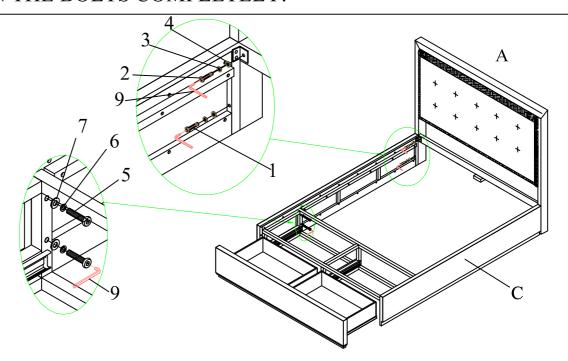
STEP 2: REPEAT STEP ONE FOR THE SECOND SIDE RAIL. TIGHTEN ALL ALLEN BOLTS FROM STEP 1 AND 2 COMPLETELY WITH THE ALLEN KEY (9).
