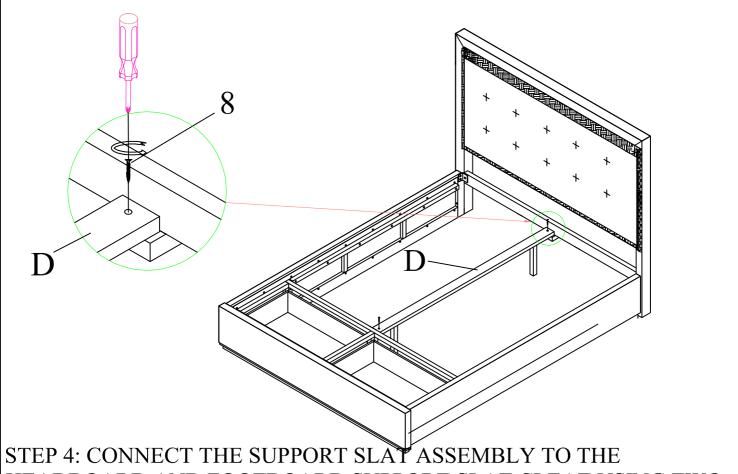
STEP 4: CONNECT THE SUPPORT SLAT ASSEMBLY TO THE HEADBOARD AND FOOTBOARD SUPPORT SLAT CLEAT USING TWO WOOD SCREWS (8).
