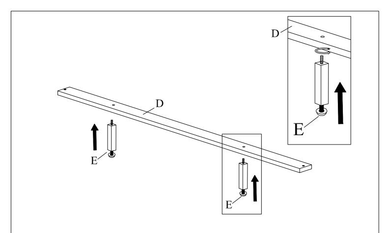
STEP 3: ATTACH THE SUPPORT LEGS (E) TO THE SUPPORT SLAT (D).
