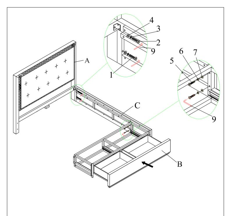
STEP 1: FOLLOWING THE ILLUSTRATION, ATTACH ONE SIDE RAIL (C) TO THE HEADBOARD (A) USING ONE M8X20 ALLEN BOLT (2), M8 SPRING WASHER (3) AND M8 FLAT WASHER (4) THROUGH THE METAL 'L' BRACKET. USE ONE M8X50 ALLEN BOLT (1), M8 SPRING AND M8 FLAT WASHER THROUGH THE WOODEN SIDE RAIL SUPPORT. DO NOT TIGHTEN THE BOLTS COMPLETELY.
