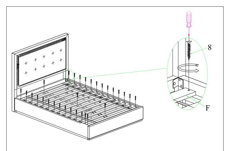
STEP 5: FOLLOWING THE ILLUSTRATION, PLACE AND CONNECT THE SLAT ROLL (F) TO THE BED WITH THE PROVIDED WOOD SCREWS.
