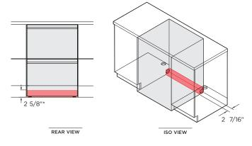
Service outlet at rear extends both sides, hoses and cords can be routed to either or both sides. Units shown in inch.
