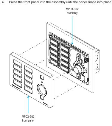
5. Test the buttons to ensure that they can be pressed and released without becoming impeded by the front panel, and test the volume knob by rotating it gently. If any buttons are impeded or if the knob does not rotate easily, remove the panel as described in step 7, adjust the button and front panel placement, and then reattach the front panel.
