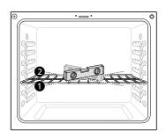
If the level doesn't show that the rack is level, adjust the leveling legs with a wrench.
