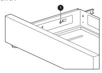
Locate the glide lever on each side of the drawer. Push down on the left glide lever and pull up on the right glide lever.
