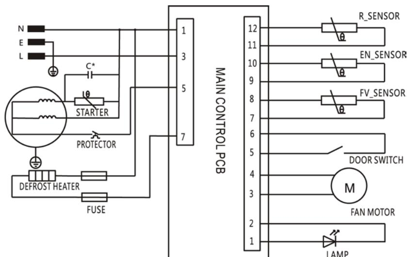
C\*:The capacitor is optional according to different compressor model
