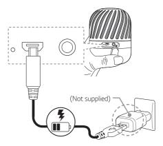
If the battery is fully charged in charging mode, Battery LED is changed from red to green. After 15 seconds, Battery LED turns off.
