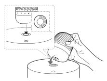
Press the speaker for fitting its hole to center of woofer station.
