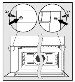
Open the door and use the screws supplied to secure the oven to the side walls of the cabinetry through the holes in the oven trim. Please have the model and serial number of your appliance available when contacting Customer Service.
