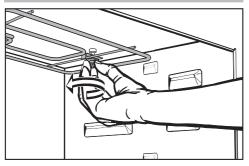
Unscrew the nut and lower the Browning / Broiling element. Use caution not to damage the Browning / Broiling element. Do not use force to lower the Browning / Broiling element.
