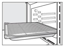
We recommend using the rack together with the glass tray when cooking items on the rack which might drip.
