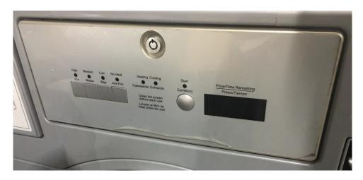
2. Remove the front control panel frame by removing the four screws shown.
