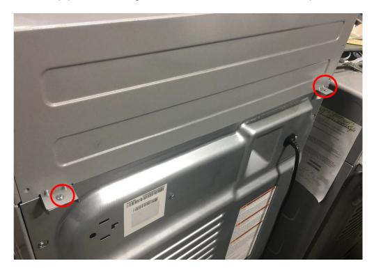
5. Slide the top cover panel forwards and then up to remove the top cover panel from the machine.
