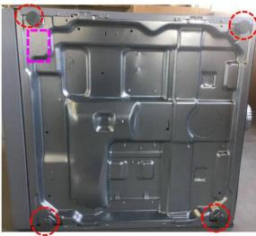
10. Remove the four adjustable feet from the dryer and remove the rectangular "knockout" plate as indicated in the picture. Loosen slightly, but do not remove, the 4 shouldered self-extrusion screws which are already attached under the base panel of the DLHS dryer.
