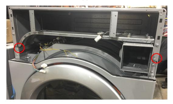
4. Remove the 2 top panel-securing screws located at the back of the panel.
