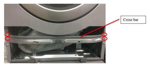
14. Feed the hex head screw previously removed in step #8 through the base of the upper machine and feed back into the threaded hole in FRONT-RIGHT mounting bracket of the lower machine using a socket ratchet, locking the position of the two machines relative to each. WARNING: This step must be done correctly to prevent the upper machine from being pushed backwards. Note: for COIN metered machines see step 16.
