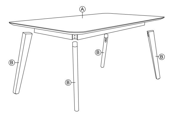
STEP 1 : Place the table top (A) upside down on a flat and clean surface. Assemble the table leg (B) to the table top (A) by using the Allen Key (4) and the hardware Bolt 5/16" x 3 3/16" (1), Spring washer (2) & Flat washer (3).
