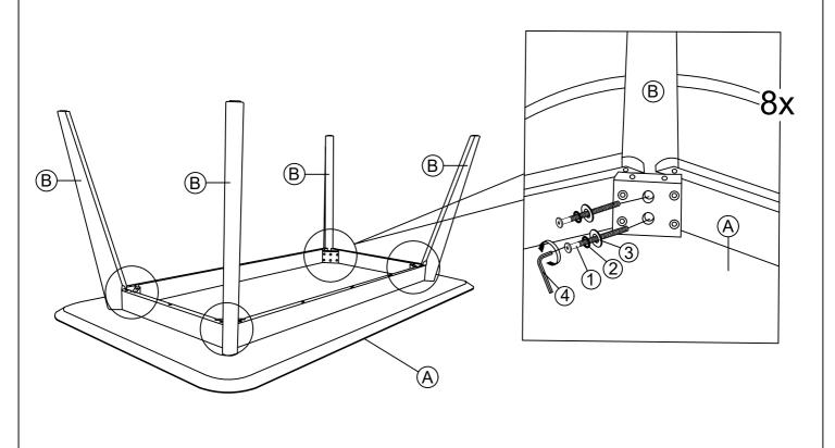
STEP 2: To level the table, stand the table upright on a flat surface and tighten all the bolts by using Allen Key (4).
