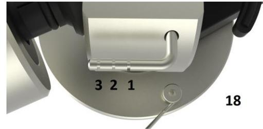
Slip the loop of the anti-skating weight's thread over the third groove of the stub to set the correct anti-skating force for the factory-fitted cartridge. Feed the thread through the loop of the wire support (17).
