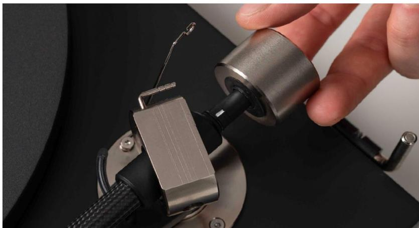
Pushing carefully, move the counterweight (6) onto the rear end of the counterweight support rod as shown in the picture below.
