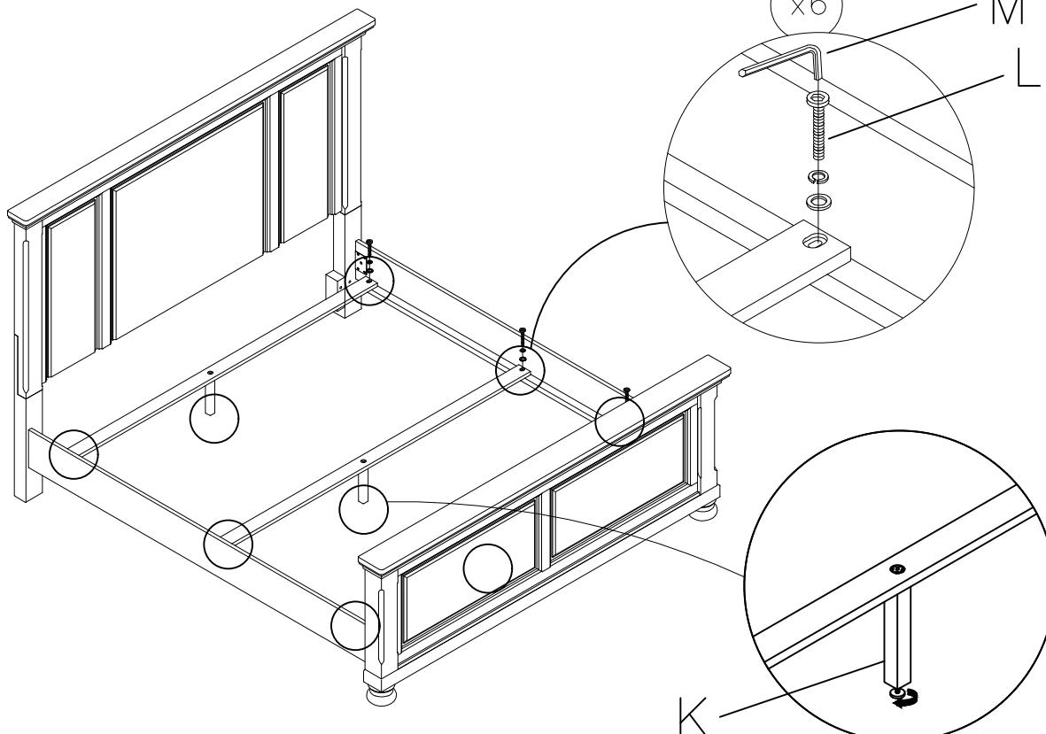
Turn Adjustable Leveler on the bottom of the Cross-Slat Support Leg leaving 6mm space between leveler and the floor.
