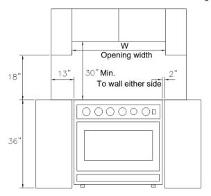
30" Model 30" (762mm) 36" Model 36" (914mm) 48" Model 48" (1219mm)
