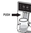
After installation or when replacing the water filter, dispense at least 1 gallon (2~3minutes) of water to remove trapped air from the water line. Otherwise, water may drip after dispensing water. (On some models)
