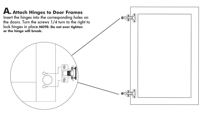
Note: The hinge can be separated by pulling the black tab and pulling apart the hinge from the hinge base. Separated hinges snap back together.
