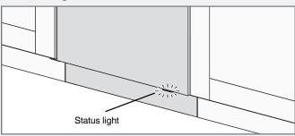
The status light at the bottom on the dishwasher provides information by means of 3 different colors.
