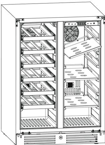
3. Pull the shelf outward until it is removed from the inner compartment. You may encounter some resistance from the shelf guard rail.
