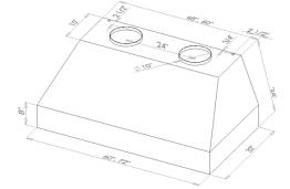
C. Duct Cover (included for ceilings from 9' to 10') c
