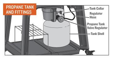
The Flat Top Grill can be used with any standard 20 lb (9 kg) propane tank. It must be a maximum of I2 I/4" in diameter; I8" high, and with right-handed connection threads. The tank must be marked in accordance with the latest U.S. Department of Transportation specifications for LP gas tanks or DOT. CFR49 or National Standards of Canada CAN/CSA-B359 Cylinders, Spheres and Tubes for the
