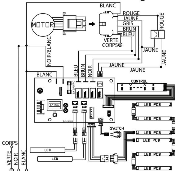
REMARKS:CONDENSER 12.5+12.5uF 250VAC FIT AC120V 60Hz
