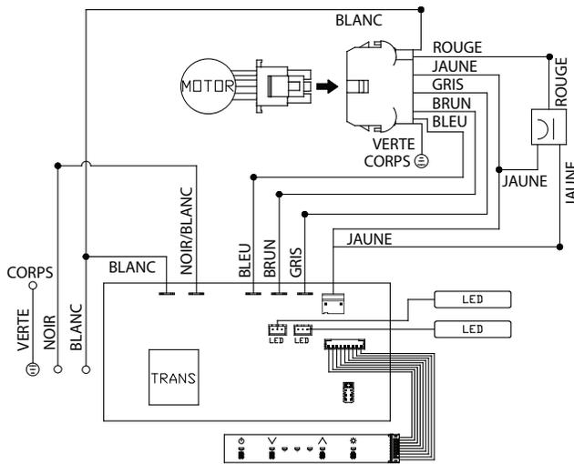
REMARKS:CONDENSER 12.5+12.5uF 250VAC FIT AC120V 60Hz
