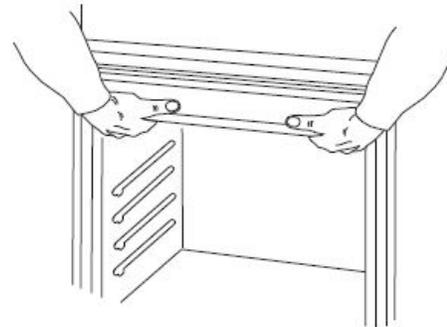
2. Push against the seal area of the front frame to push the oven into the cabinet until the back surface of the front frame touches the front wall of the cabinet.
