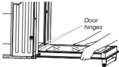
3. Locate the oven door hinge locks in both corners of the oven door, and rotate the hinge locks toward the oven door to the unlocked position. If the door hinge lock is not rotated fully (see illustration B), the door will not remove properly.
