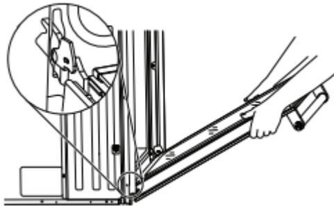
**IMPORTANT:** Do not close the door at this step or damage may occur to the door hinge.
