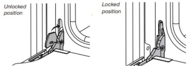
7. After the door hinges have been locked, gently swing the door upward to close. The door should not be forced closed.
