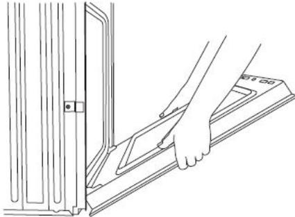
5. Using 2 hands, grasp the edges of the oven door. Close the oven door slightly past the stop position to take the weight off of the door hinges, and then pull the oven door up.
