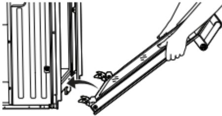
4. Make sure the door hinge notch is engaged on the bottom of the oven cavity slot.
