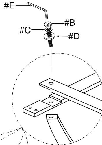
Align stretchers (#3,4) to the legs, then secure by using bolts (#B) with washers (#C,D).
