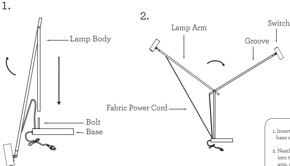
1. Insert the lamp body onto bolt of lamp base and ensure it is secure.
