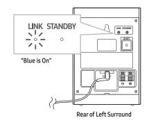
If the LINK LED does not turn to solid blue in a minute, please repeat from step 2 through 5 referring to step 6
