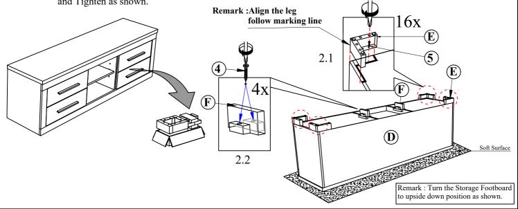
**STEP 3.1**: Pull the drawer and take out the Leg (I),(J)&(K). Attach the Chrome metal leg (I) at the bottom Storage side rails (H). Used Pan head chipboard screw(5) and Tighten as shown.
