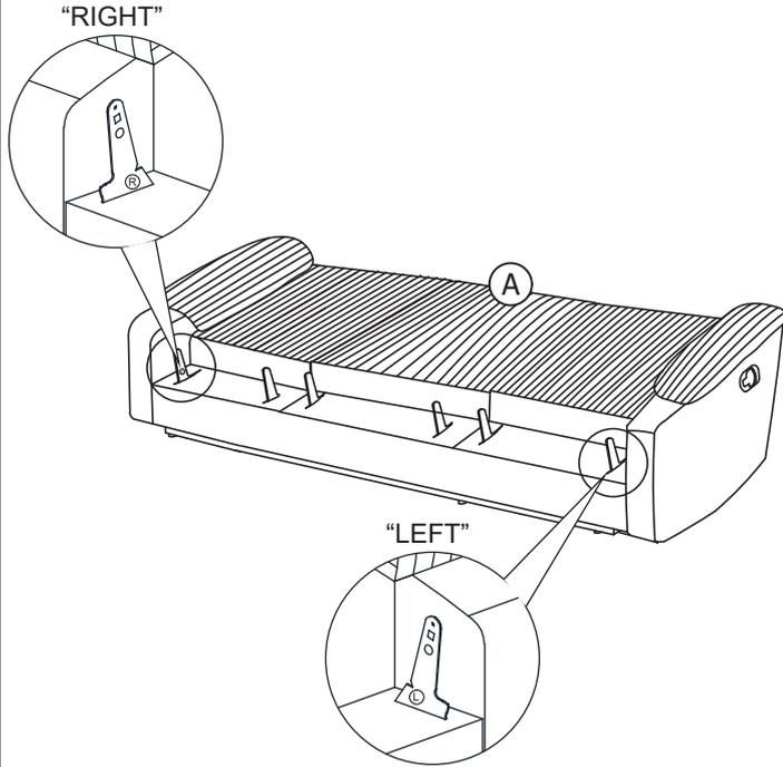
**STEP 2:** Install the backrests (B/C/D) by align and insert the metal bracket on the backrests (B/C/D) to the metal bracket of the seat (A). Please make sure the brackets are inserted all the way and secured into position.
