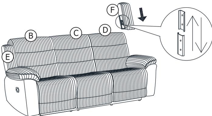
**STEP 4:** Press the Velcro strip on the backrests (B/C/D) to the Velcro strip on the bottom of seat (A).
