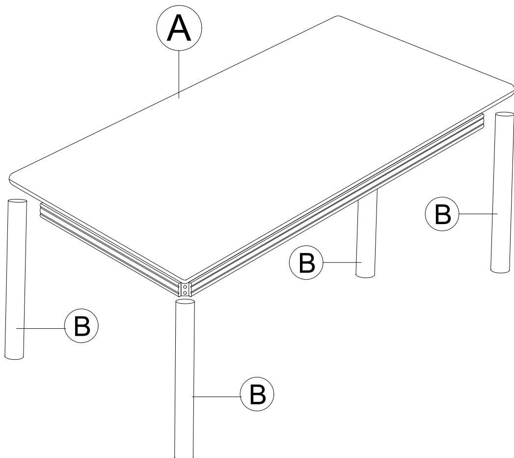
STEP 1 : Place the table top (A) upside down on a flat and clean surface. Assemble the table leg (B) to the table top (A) by using the Wrench (4) with hardware Hex Com Bolt 5/16"x 2" (1), Spring washer (2), and Flat washer (3).
