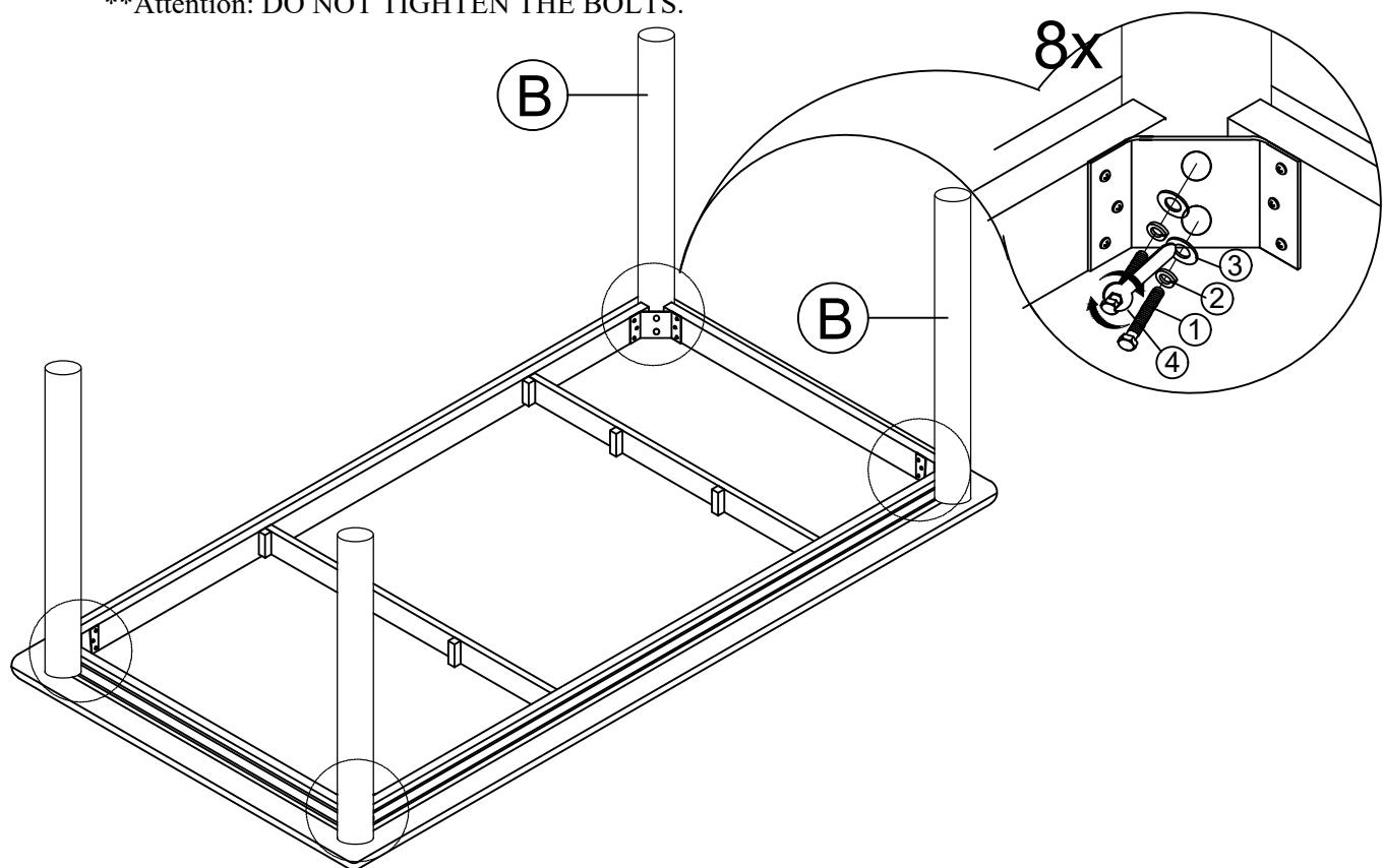
STEP 2 : To level the table, stand the table upright on a flat surface and tighten all the bolts by using Wrench (4).
