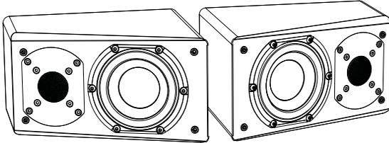
**Bipole Mode** - Bipole mode is recommended for home theater systems which have a 7.1 AV receiver and use dedicated side surround and rear surround speakers. In bipole mode, both sets of speakers have the same output, which is "in phase". This will provide a more localized and directional surround sound effect.
