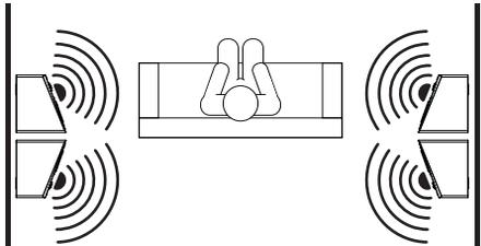
**Dipole Mode** - In dipole mode, one Elevation speaker is electrically reversed from the other, or "out of phase." This will provide a more diffuse and non-directional surround sound effect.
