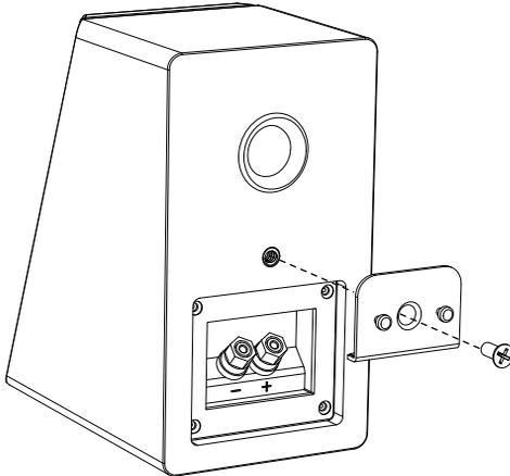
5) Connect the speaker wire to your binding posts and hang the Prime Elevation on the Multi-Angle Wall Bracket (patent pending) as shown. The foam gasket will make a tight fit and reduce any possible vibration noise.
