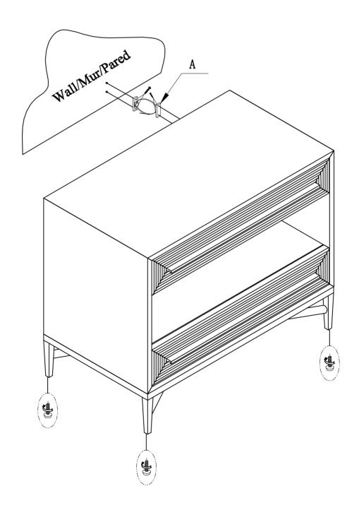
Adjust levelers if needed, to level case on uneven floor
