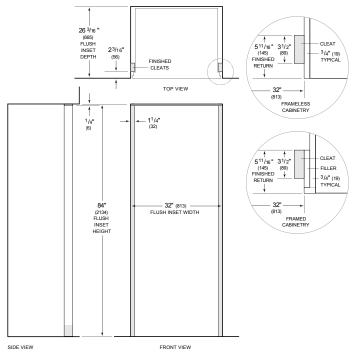
NOTE: 31/2" (89) finished returns and shaded areas will be visible and should be finished to match cabinetry Shaded line represents profile of unit **b**it/1/4" (19) panel.
