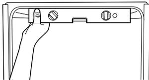
2. Use the level to check if the dishwasher is level front to back, as shown in the figure to the right. If the dishwasher is not level front to back, adjust the height of the rear leg until the dishwasher is level. See the second note below for instructions on adjusting the rear leg.
