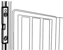
3. Open the door of the dishwasher and check if both the tub and door clearances are correct. If not, rotate the leveling legs on the bottom front of the dishwasher. You can also check this by placing a level against an inside front vertical surface of the tub.
