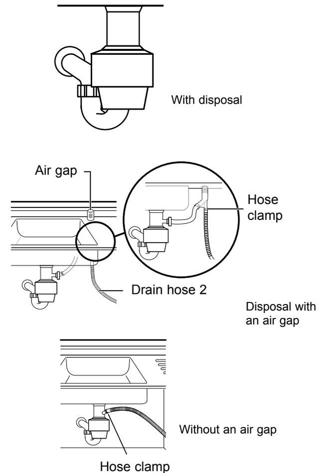
3. Check the size of the sink's drain hose connector (21 mm- as shown in Figure 8 below). If the end of the drain hose does not fit onto the drain hose connector of the sink, use an adaptor purchasable at a plumbing/hardware supply store.
