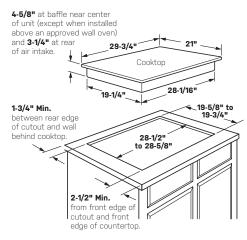
To ensure accuracy, it is best to make a template when cutting the opening in the counter.
