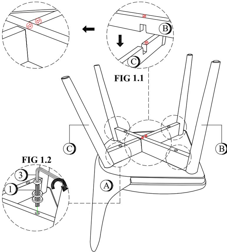
**Step 1.1** Attach Upper Leg Frame (B) and Lower Leg Frame (C) to Cushion seat (A) as shown on FIG 1.1
