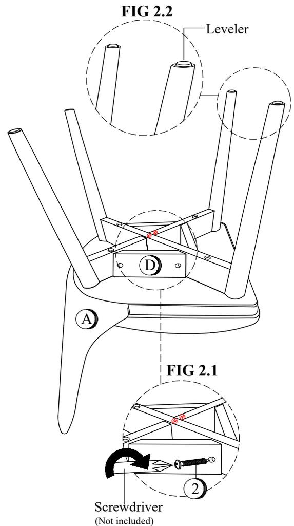
**Step 2.1** Insert Screw (2) through Corner block (D) into Leg Frames (B, C) as shown on FIG 2.1
