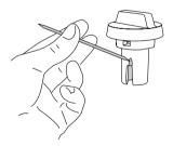
(5) Wash all the components of the frother thoroughly with hot water and dishwashing liquid. All components and the container are dishwasher safe. Make sure there are no milk residues on the hollow and groove under the dial. If necessary, scrape the groove with a toothpick.
