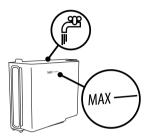
③ RINSE AND FILL WATER TANK UP TO MAX LEVEL: the appliance is now ready to rinse with fresh water. Empty the container used to collect the descaler solution. Remove the water tank, rinse under running water, fill with fresh water up to the MAX level and put back in the appliance.
