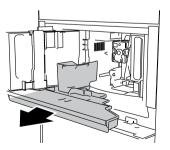
(6) EMPTY GROUNDS CONTAINER AND DRIP TRAY: remove, empty and replace the drip tray and grounds container. Press NEXT.
