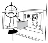
When EMPTY GROUNDS CONTAINER appears on the display, the grounds container must be emptied and cleaned. The appliance cannot be used to again until you have cleaned the grounds container. Even if the container is not full, the empty grounds container message is displayed 72 hours after the first coffee has been prepared. For the 72 hours to be calculated correctly, avoid turning the appliance off from the mains switch if it is not necessary. To clean (with the appliance on):
