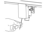
(2) Check that the holes in the coffee spouts are not blocked. If necessary, remove coffee deposits with a toothpick.
