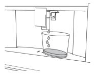
PLACE 2L CONTAINER UNDER SPOUTS PRESS TO START DESCALING: Place an empty suitably sized container under the steam wand and coffee spouts.
