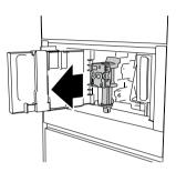
(4) Press the two coloured release buttons inwards and at the same time pull the infuser outwards.
