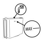
INSE AND FILL WATER TANK UP TO MAX LEVEL: Fill the tank up to the MAX level with fresh water.
