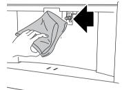
Remove the milk container and clean the steam connection nozzle with a sponge.
