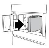
INSERT WATER TANK: Place the water tank back in the appliance.
