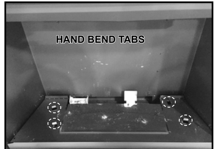
Figure 3. Hand Bend Tab Locations - QUARTZ36 Shown
