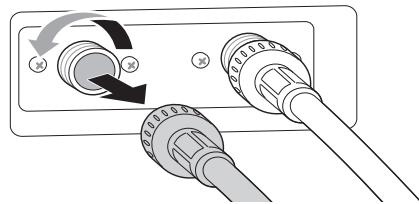
**7** Insert the drain pump filter and twist it clockwise.
