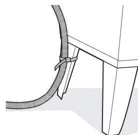
**4** If the water valves and drain are built into the wall, fasten the drain hose to one of the water hoses with the provided tie strap (3) (ribbed side on inside).
