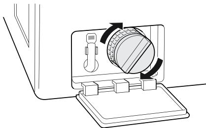
**8** Close the drain pump filter cover.
