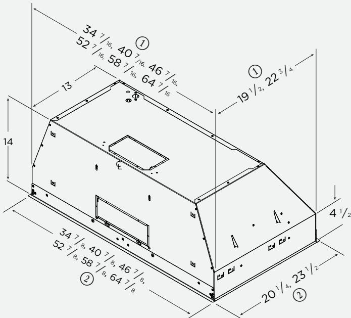
**Note:** Specification drawing dimensions and cutout dimensions assume the use of all four trims around the unit. **Front and back trims can be removed. Side trims are not removable.**
