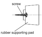
3. Make screw in alignment with the hole on lower base cover. Fasten rubber supporting pad to the base cover firmly by a cross screwdriver (self-provided).
