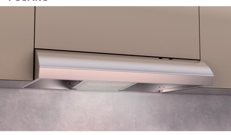
Fusaro has a slender 5" height and soft curves, designed to modernize and perfectly fit kitchens where space is premium. A 2-speed, 190 CFM internal blower provides sufficient ventilating power for most kitchens. Color coordinated rocker switches control blower speeds and 75 Watt incandescent lightning. The anodized aluminum mesh grease filter is dishwasher safe and simple to remove and re-install. Fusaro is designed for standard ducted installation ONLY.
