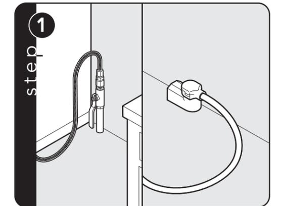
Connect gas and electrical. Before placing appliance in operation, always check for gas leaks. This must be performed by your dealer, a qualified licensed plumber, or gas service company.
