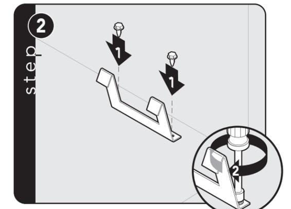
Mount anti-tip bracket hook to floor using screws provided.
