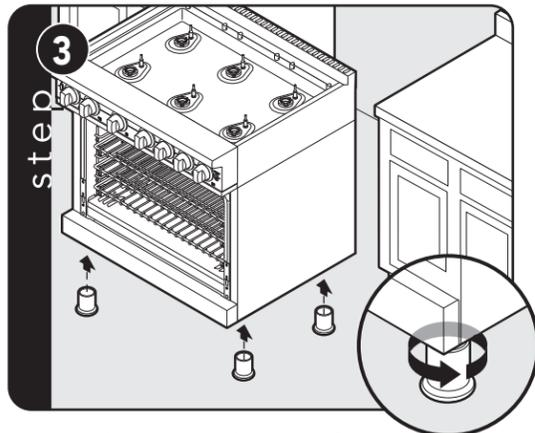
Screw legs into couplings on all four corners. The 48" W. ranges have two additional legs located in the center of the unit.
