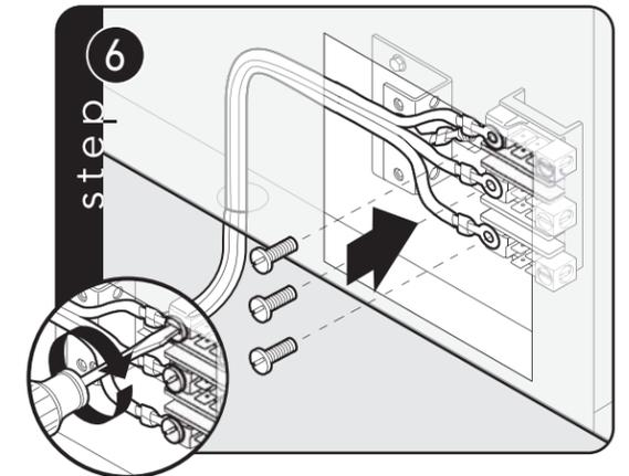
Attach line #1 (red) and line #2 (black) leads to outside terminals. Attach neutral wire (white) to center terminal on terminal block.
