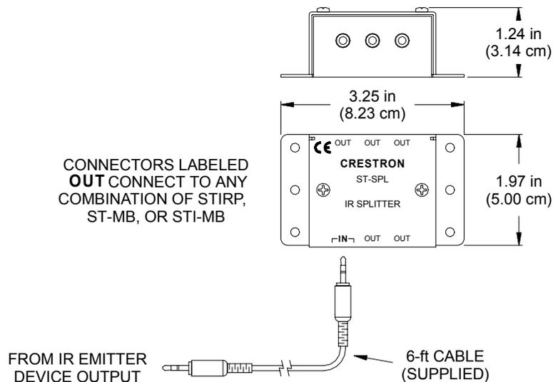
The ST-SPL enclosure extends to form mounting flanges at the sides of the unit. There are three holes per flange for installing screws (not supplied) to mount the unit.
