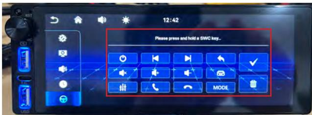
After properly connecting the steering wheel control wires, press the desired button on the steering wheel, then touch the corresponding function on the screen. Repeat this step until all commands have been programmed, then tap 'confirm'.
